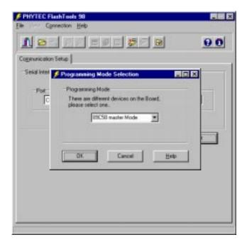
• If the *Programming Mode Selection* window appears choose *xxx external Flash* where *xxx* describes the Flash device currently mounted on the Modul.
