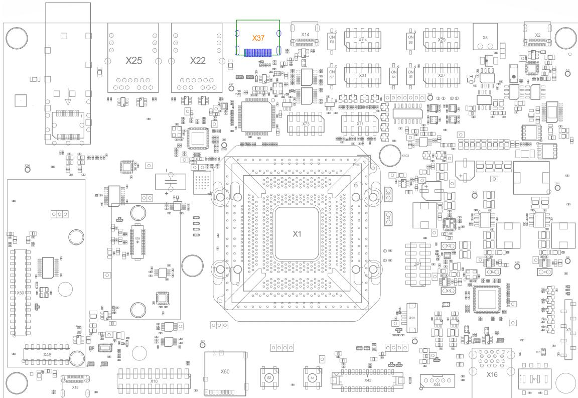
The Libra Development Board provides a High-Definition Multimedia Interface (HDMI), which is compliant with HDMI 2.0a. It supports a maximum resolution of 1920x1080p60, 1280x720p60, 720x480p60, and 640x480p60. Please refer to the applicable phyFLEX FPSC SoM Applications Processor Reference Manual for more information. This feature is not available for all mountable FPSC SoMs.
