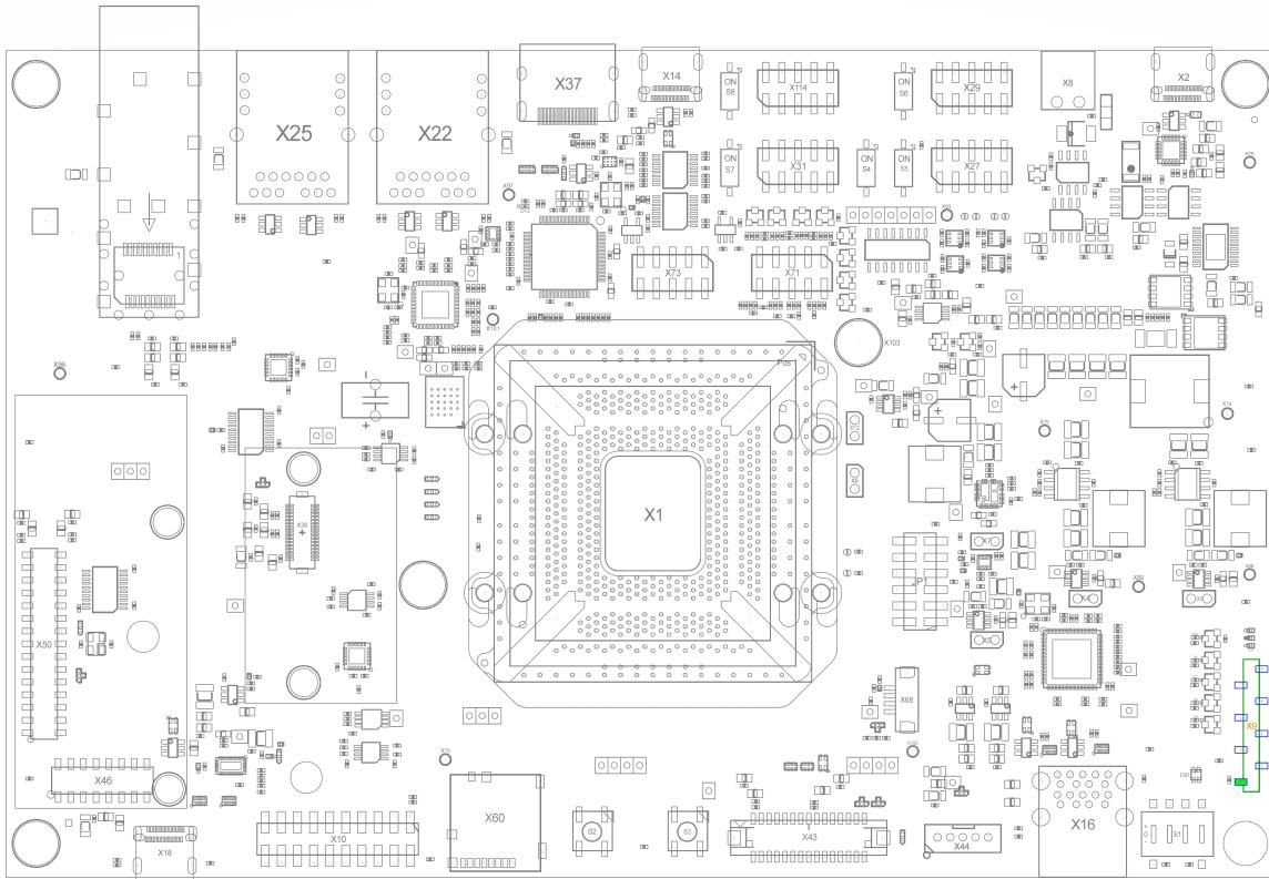
The Libra Development Board features a tri-state boot switch with four individually switchable ports to select the phyFLEX FPSC SoM default bootsource. The Boot\_Mode signals may also be accessed through pin header X9 or USB to UART/GPIO converter U15. Descriptions of the various boot modes can be found in [Boot Mode Selection](#). The available boot options differ depending on the mounted phyFLEX SoM. All available options are displayed in the
