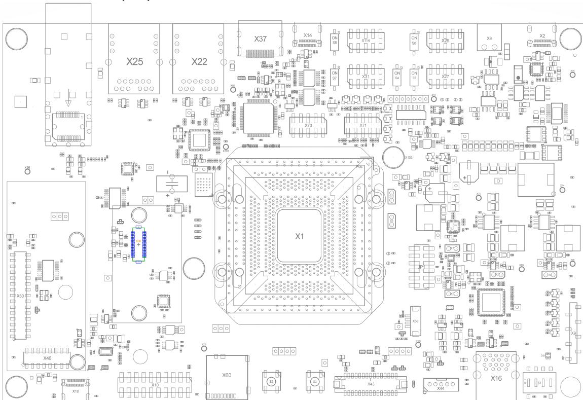
The Libra Development Board offers one MIPI-DSI display interface. MIPI-DSI has 4 channels, supporting one display with a resolution of up to 1920 x 1080 at 60Hz. The following table shows the pin assignment of connector X39. This feature is not available for all mountable FPSC SoMs.
