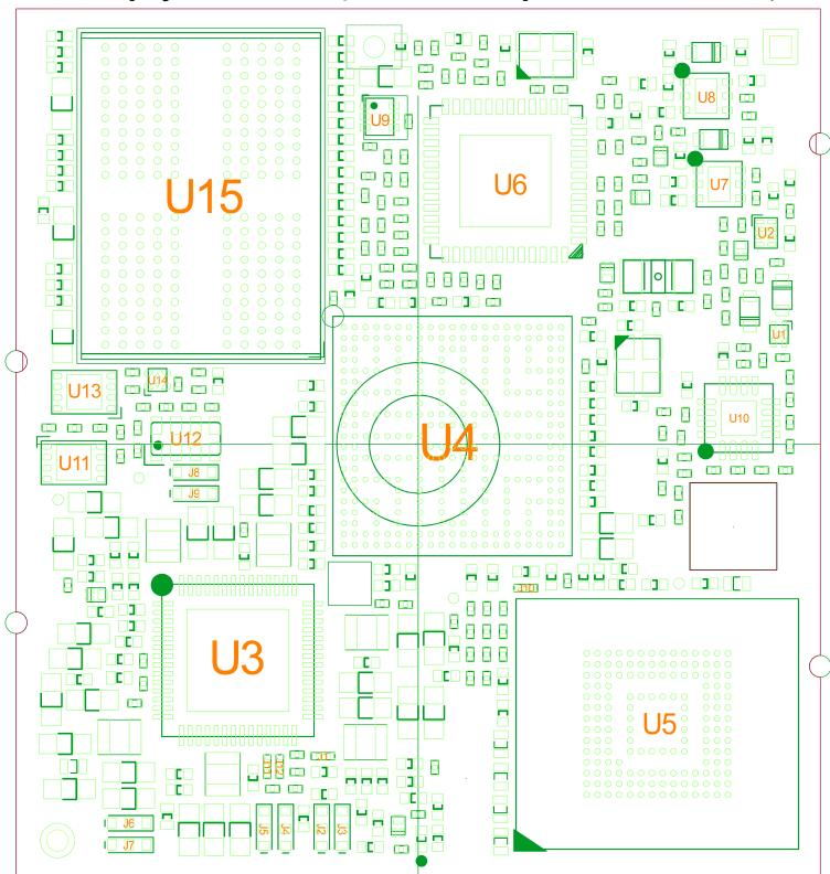
**FIGURE 3: phyFLEX-i.MX 91/93 FPSC Component Placement (1634.0 Bottom View)**
