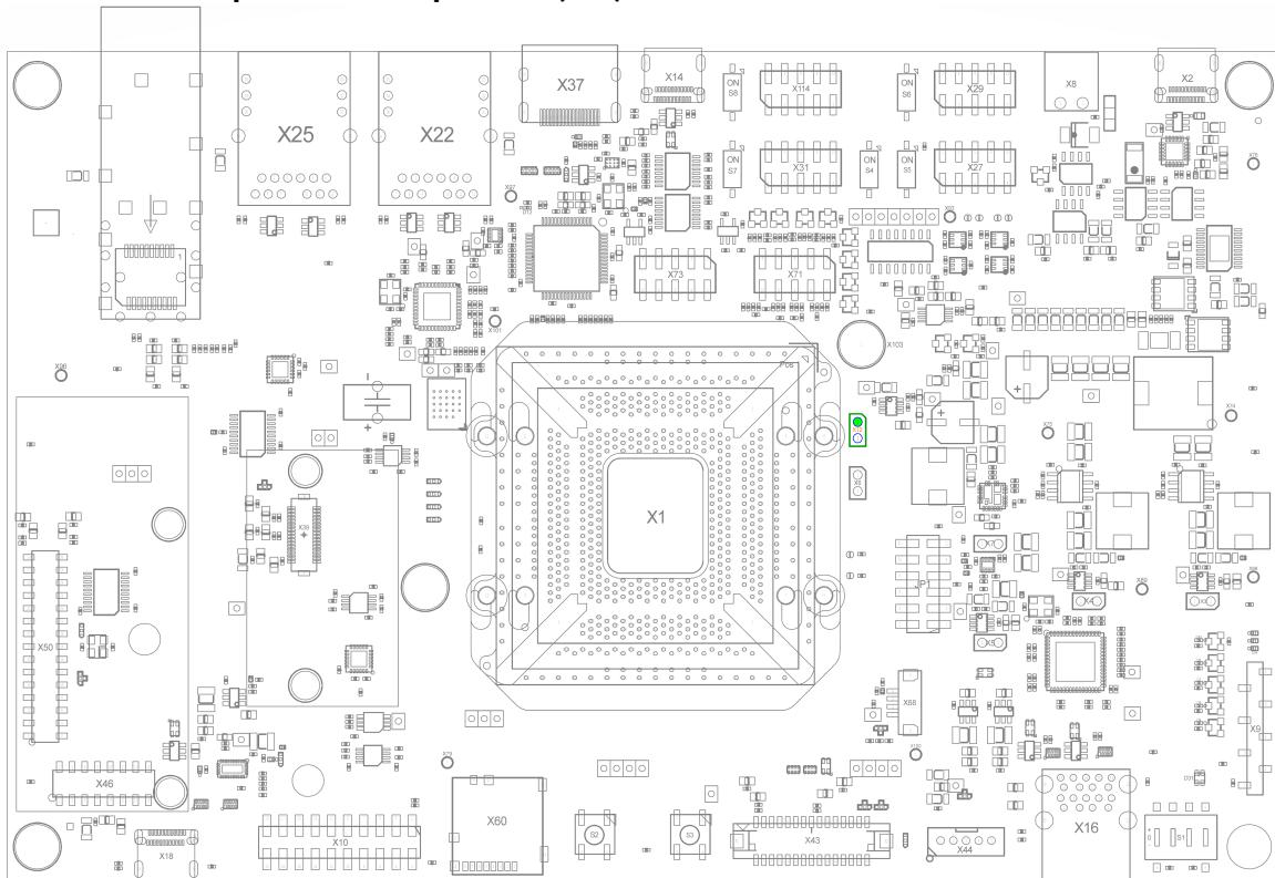
The input current of the SoM supply rail VDD\_SOM can be measured on board to determine the power consumption of the SOM. A current sense amplifier translates the supply current into a proportional voltage VOUT\_CC\_SOM, which can be measured at X12 (on PCB top side) and X12 (on PCB bottom side). The mounted amplifier features a gain of 100V/V. The SoM input current  $I_{SOM\_IN}$  in Ampere is determined by inserting VOUT\_CC\_SOM into the following equation.
