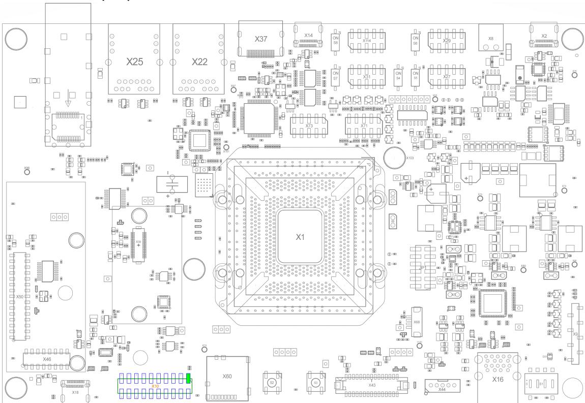
The Libra Development Board provides a 2x10 2.54mm pin-header for JTAG connectivity. 1.8 V are available at the connector directly or with a 100R pull-up.
