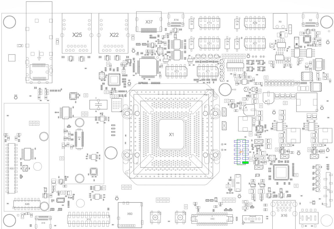
The Libra Development Board comes pre-configured with several removable jumpers (JP) and solder jumpers (J). These jumpers enable the flexible configuration of a limited number of features for development purposes.
