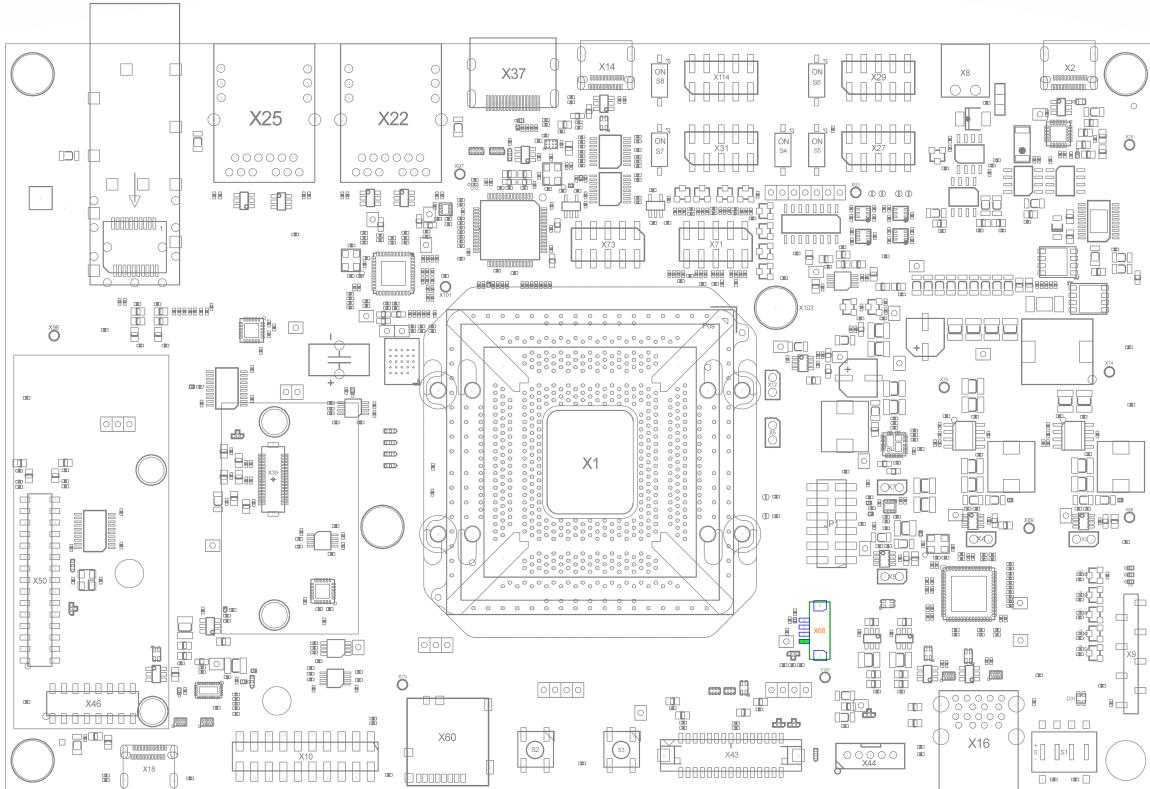
If heatsinking is required for the phyFLEX FPSC SoM, a PWM-controlled fan can be connected to the Libra Development Board. The fan's supply voltage is 5 V by default but can be changed to 12 V or VDD\_IN (carrier board input voltage) via J19. The PWM signal is brought out as open drain pulled up to VDD\_5V0 with a 4k7 resistor. The fan feedback signal, which can be used to monitor fan rotational frequency, is connected to X\_FAN\_FB and pulled up to VDD\_1V8 via a 4k7 resistor.
