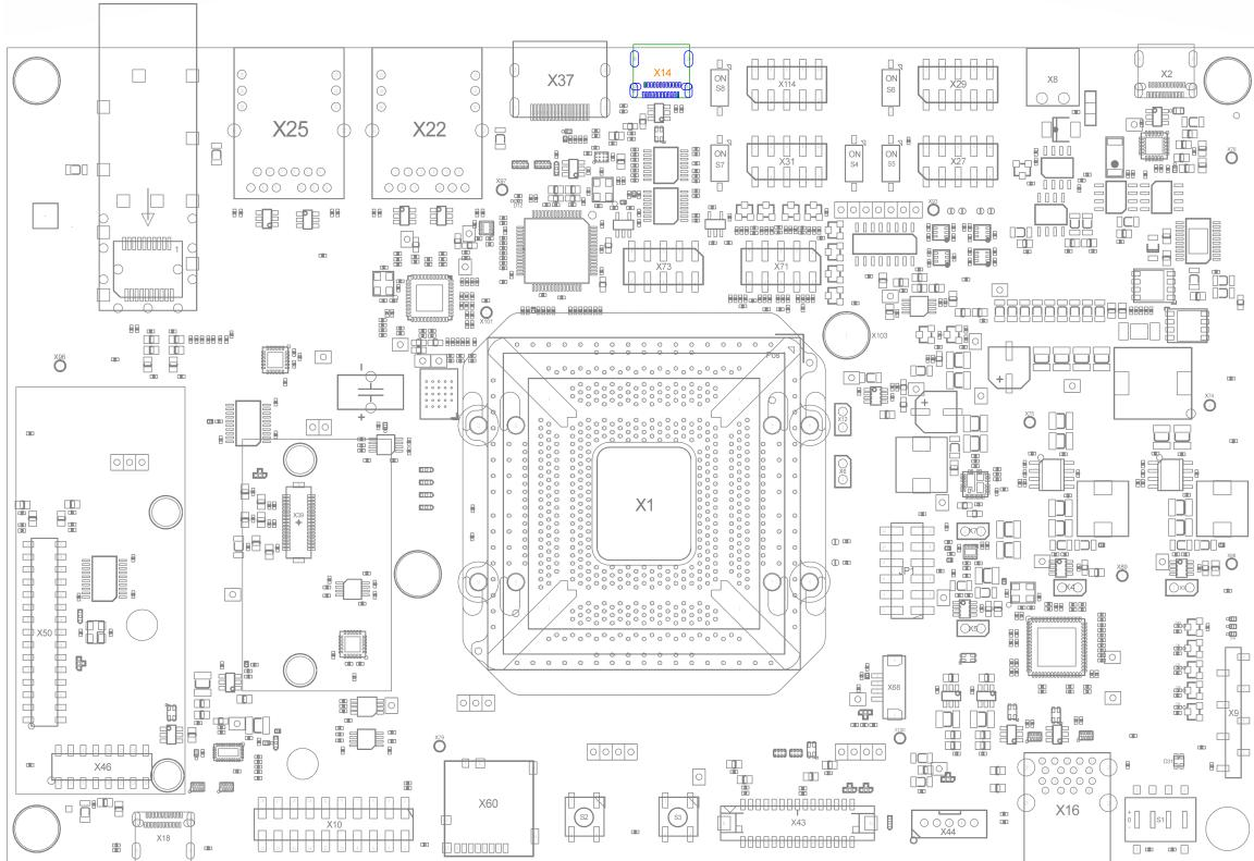
The primary debug interface is UART3. UART2 is the special debug interface used to connect to an M-core or similar provided by the SoM. Both UART interfaces are connected to a UART-to-USB converter (U15 FTDI FT4232H). The USB 2.0 interface is brought out at a USB-C socket (X14). Use the following terminal settings to connect to the Libra Development Board serial interfaces:
