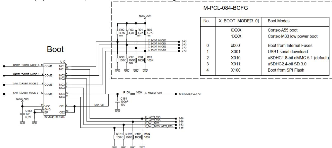
The BOOT\_MODE is initialized by sampling the BOOT\_MODE inputs on the rising edge of the X\_nRESET\_OUT. After these inputs are sampled, their subsequent state does not affect the contents of the BOOT\_MODE internal register. X\_BOOT\_MODE module input signals are connected only during the reset phase to the processor inputs. For runtime, the X\_UART and X\_SAI1 signals are routed through the MUX U10.
