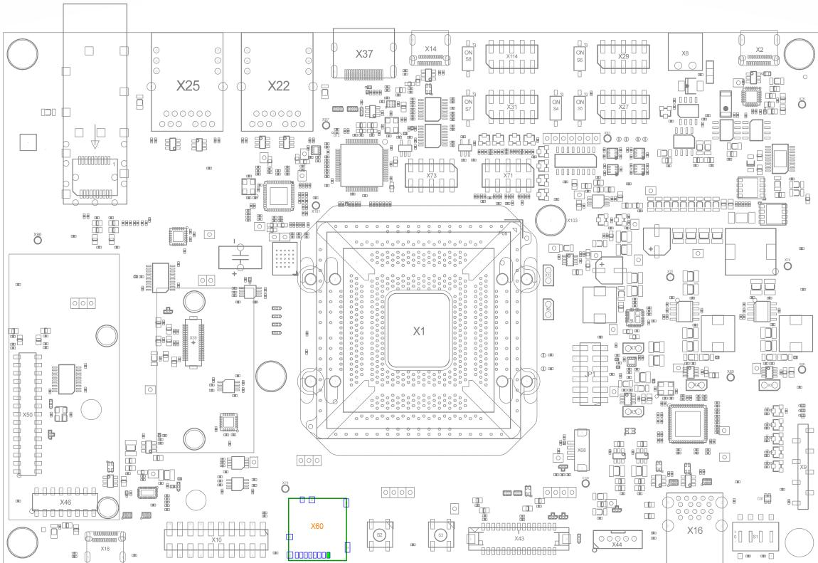
The Libra Development Board provides a standard microSDHC card slot at X60 for use with SD/MMC interface cards. It allows for a fast, easy connection to peripheral devices like microSD and MMC cards. Power to the SD interface is supplied by inserting the appropriate card into the SD/MMC connector. It also features card detection, a lock mechanism, and a smooth extraction function by pushing the card in and out.
