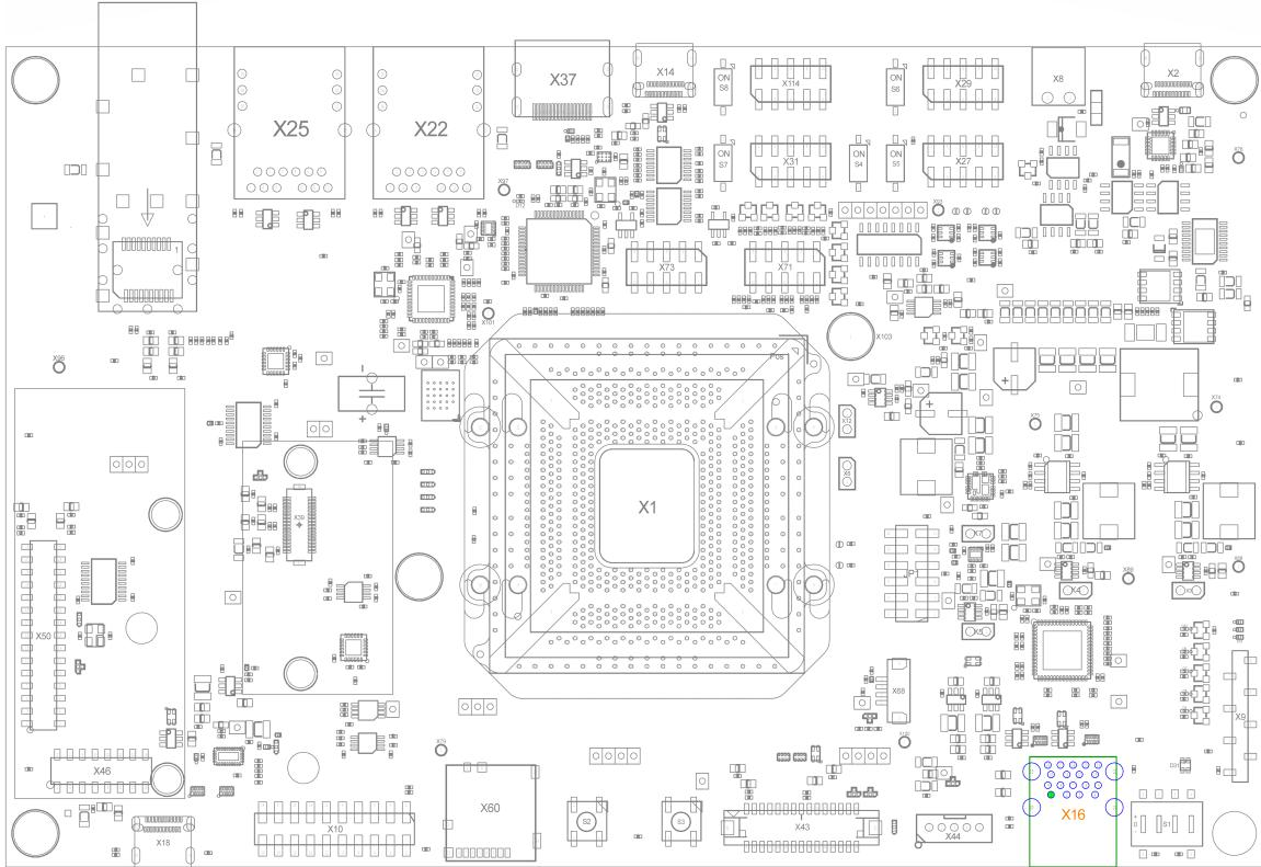
The Libra Development Board provides two USB 3.0 interfaces at the USB Dual Type-A connector X16. They are HOST interfaces made available through a 4-port USB HUB. USB1 will be at the connector's top and USB2 at the bottom receptacle.
