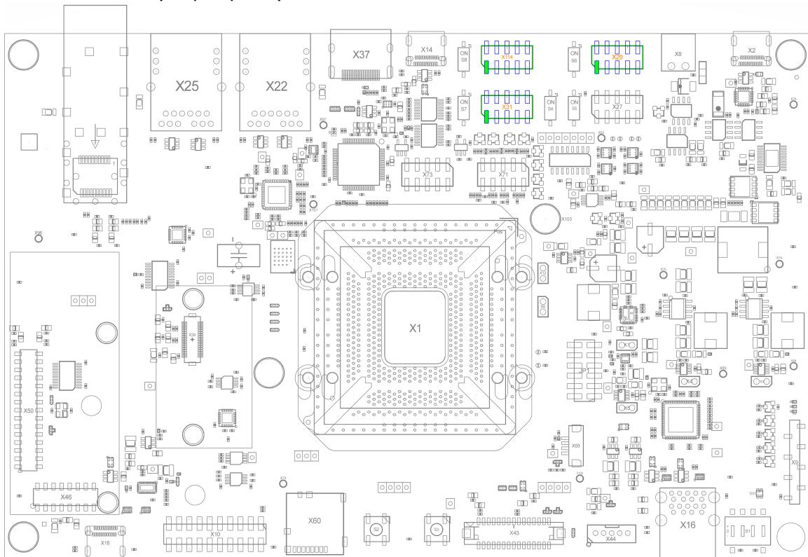
The phyFLEX FPSC SoM FLEXCAN1, FLEXCAN2, and FLEXCAN3 interfaces are brought out at X29, X31 and X114, each as CAN FD. The maximum permissible CAN FD data rate is 8 Mbit/s. For development purposes, a 120  $\Omega$  termination can be added by closing SW5 (CAN1), SW6 (CAN2) or SW8 (CAN3). For standard use, it is possible to mount a more suitable split termination in a customer-specific BOM.
