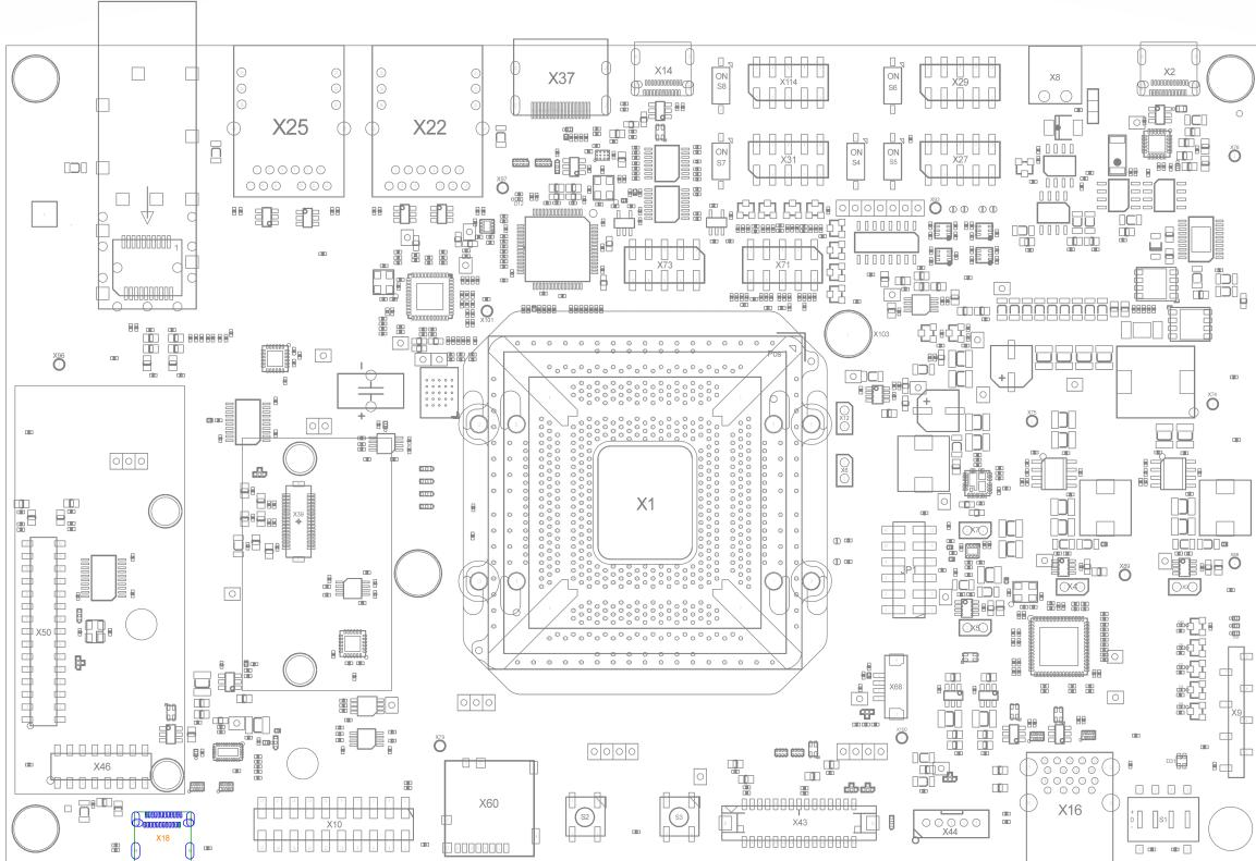
The Libra Development Board provides a USB-C 3.2 GEN 1 Dual Role interface. Muxing of super-speed differential data lanes is handled through a dedicated muxing IC (U66). The mounted SoM's USB Serial Downloader requires this interface to be able to boot from USB.
