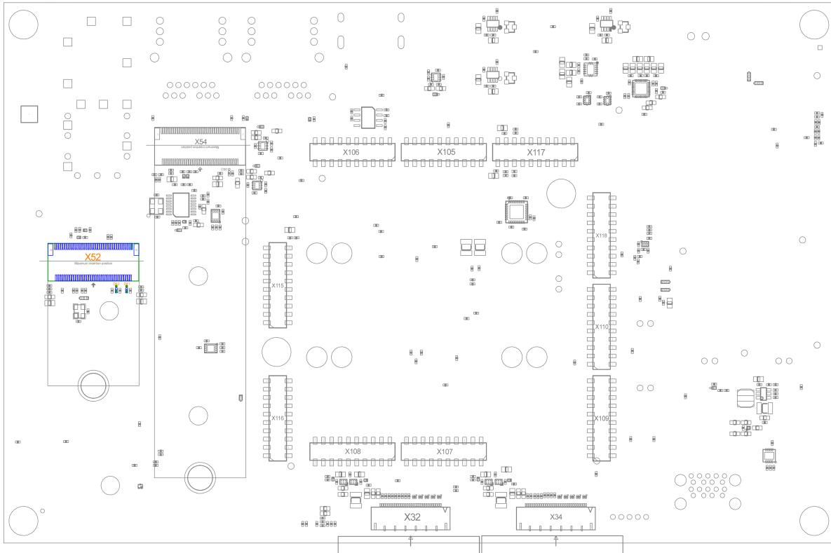
The 1-lane PCI Express interface provides PCIe Gen. 3.0 functionality, which supports up to 8 GT/s operations. Various control signals are implemented with GPIOs. The PCIE1 interface is brought out at the M.2 Key-E connector X52 shown above. The M.2 Key-E connector also features UART with flow-control, SDIO, I2C and USB 2.0.
