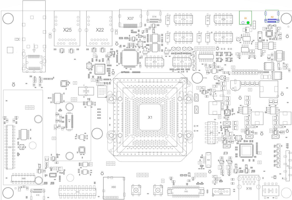
The Libra Development Board can be powered either by a 2-pole Phoenix Contact MINI COMBICON base strip 3.5 mm connector (X8) or by a USB Power Delivery Supply (X2).
