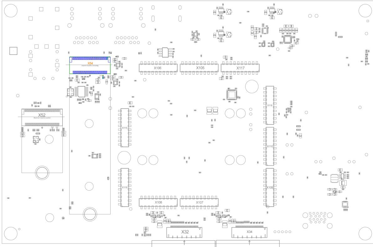
The second 1-lane PCI Express interface provides PCIe Gen. 3.0 functionality, which supports up to 8 GT/s operations. The mounted M.2 Key-M connector is mainly used for SSD cards. Various control signals are implemented with GPIOs. The PCIE2 interface is brought out at the M.2 Key-M connector X54 shown above. The PCIe clock is generated by the dedicated PCIe clock generator U51. This feature is not available for all mountable FPSC SoMs.
