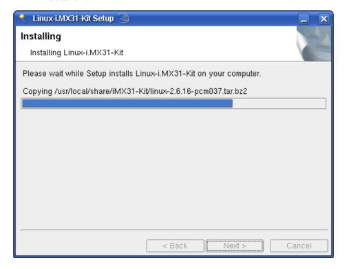
The GCC C/C++ tool chain will be installed to the default directory /opt/OSELAS.Toolchain-1.99.3/arm-1136jfs-linux-gnueabi. The program mkimage will be installed to /usr/local/bin. All other programs and examples will be installed to the selected destination directory.
