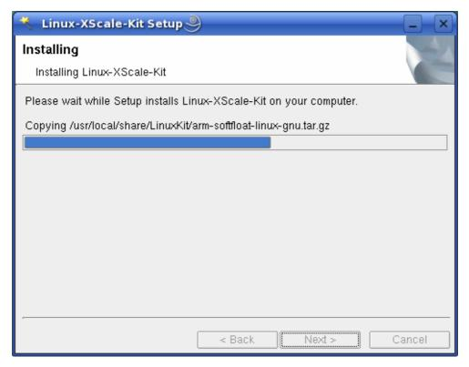
The GNU GCC C/C++ Toolchain will be installed to the standard default directory /opt/arm-softfloat-linux-gnu. The program mkimage will be installed in /usr/local/bin. All other programs and examples will be installed in the selected destination directory.
