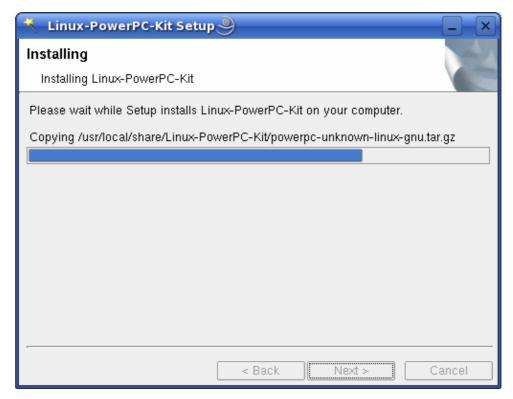
The GNU GCC C/C++ Toolchain will be installed to the standard default directory /opt/powerpc-unknown-linux-gnu. The program mkimage will be installed in /usr/local/bin. All other programs and examples will be installed in the selected destination directory.
