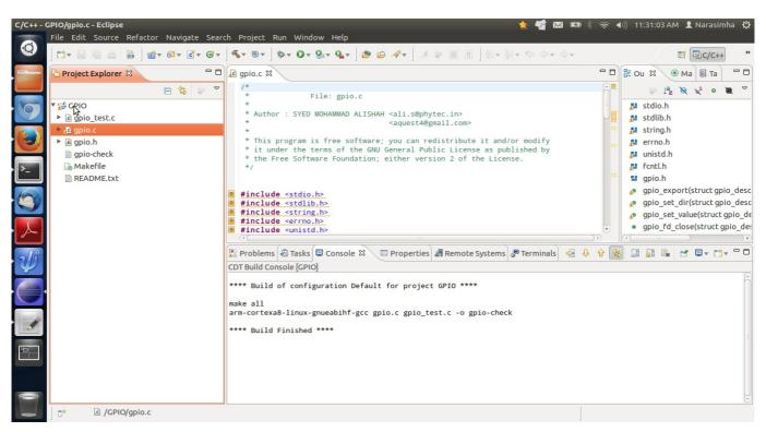
4. Right-Click on GPIO from Project-Explorer & select Run-As(from Drop-Down-Menu). Then, do settings and below: [Note: Connection:WEGA, Project:GPIO & C/C++ Application:gpio-check etc.,]
