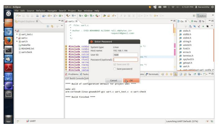
4. Right-Click on UART from Project-Explorer & select Run-As(from Drop-Down-Menu). Then, do settings and below: [Note: Connection:WEGA, Project:UART & C/C++ Application:uart-check etc.,]
